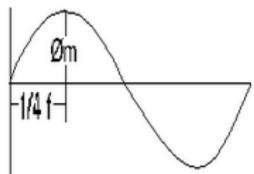
The flux increases from it's zero value to maximum value om in one quarter of the cycle i.e. in 1/4 f second.
